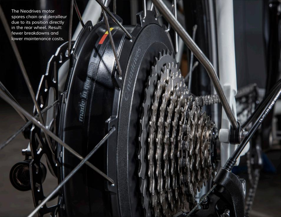
The Neodrives motor spares chain and derailleur due to its position directly in the rear wheel. Result: fewer breakdowns and lower maintenance costs.
